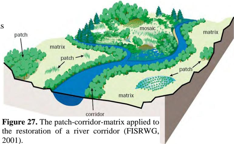
**Figure 27.** The patch-corridor-matrix applied to the restoration of a river corridor (FISRWG, 2001).
